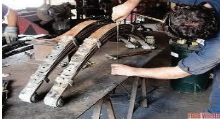
Fig.3.2 manufacturing of a leaf spring
