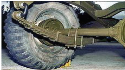
Fig.1.1 A traditional leaf spring arrangement.
